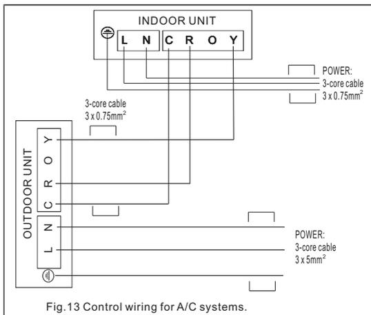
Fig.13 Control wiring for A/C systems.
